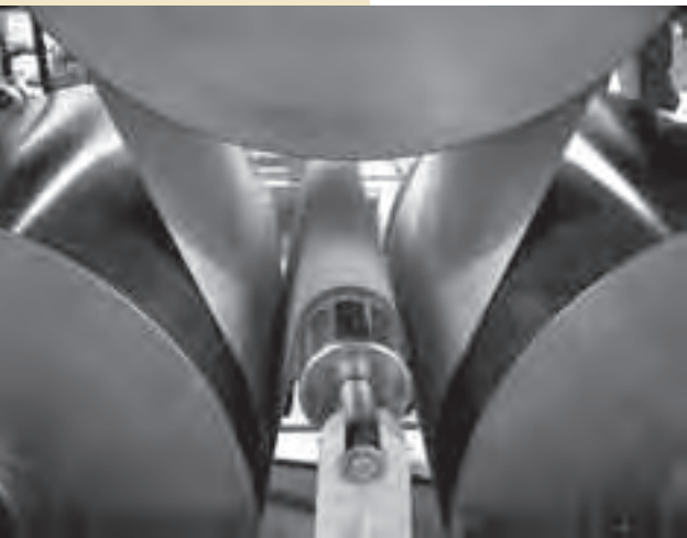
Paper from Leopold pine pulp is dried into sheets by heated rollers at the UW-Stevens Point Paper Science Lab.
