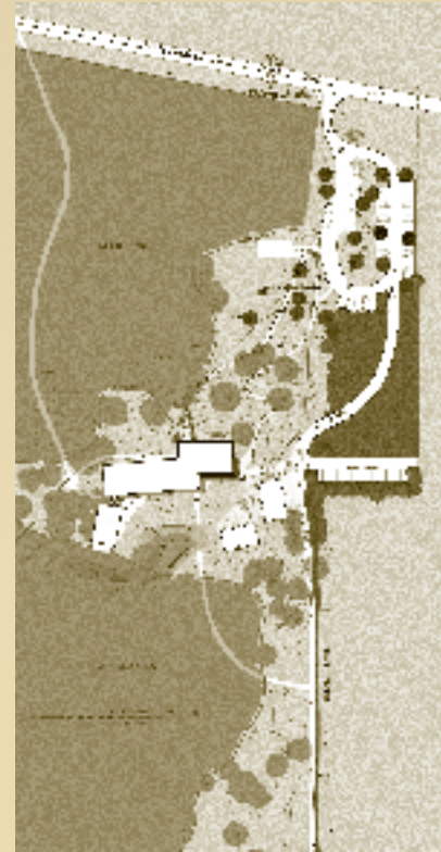
Site Plan: A small campus minimizes the visual impact of the Legacy Center and allows various functions to be isolated in order to optimize the heating and cooling requirements.
